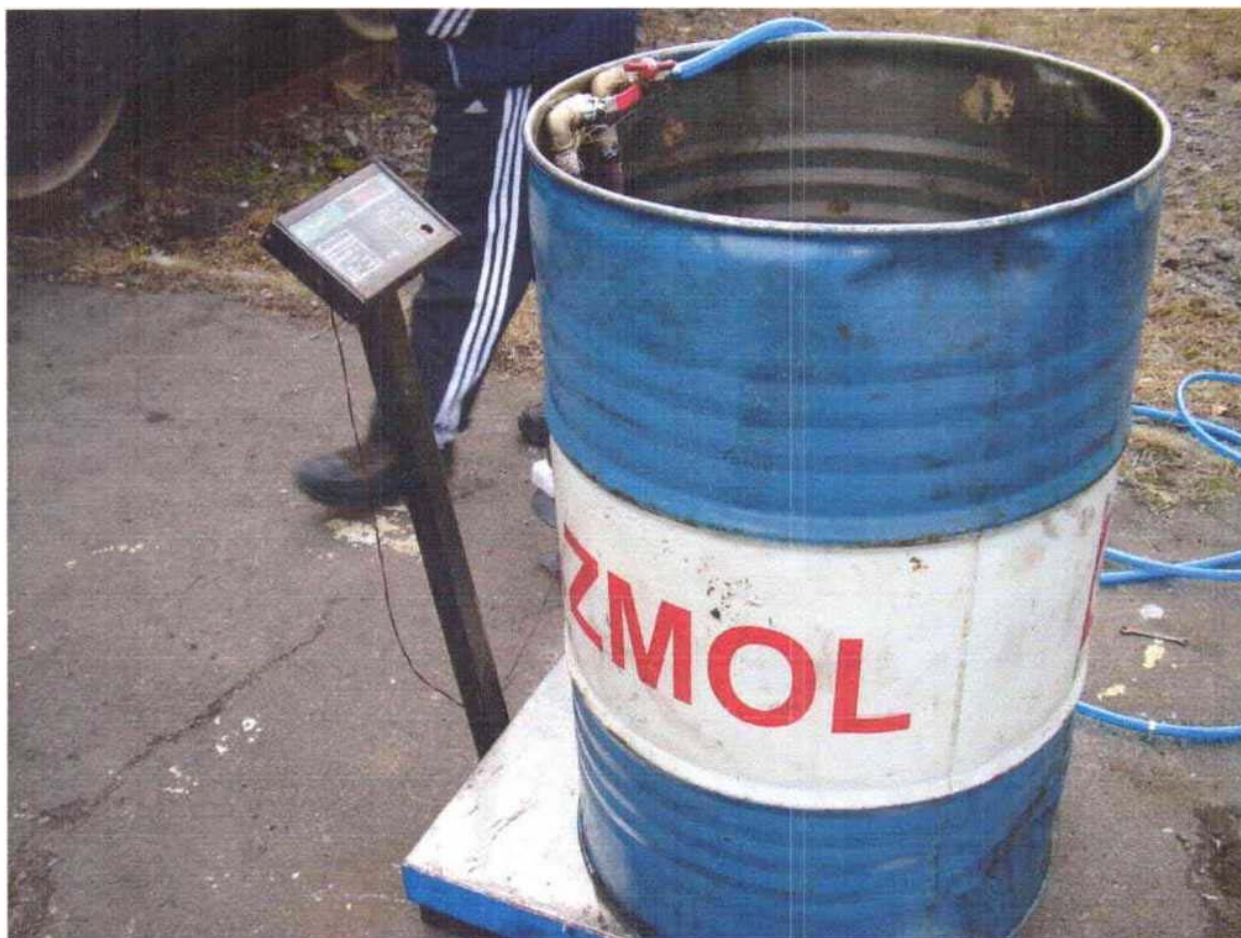
Photo 4. Tank with fuel on the scales
